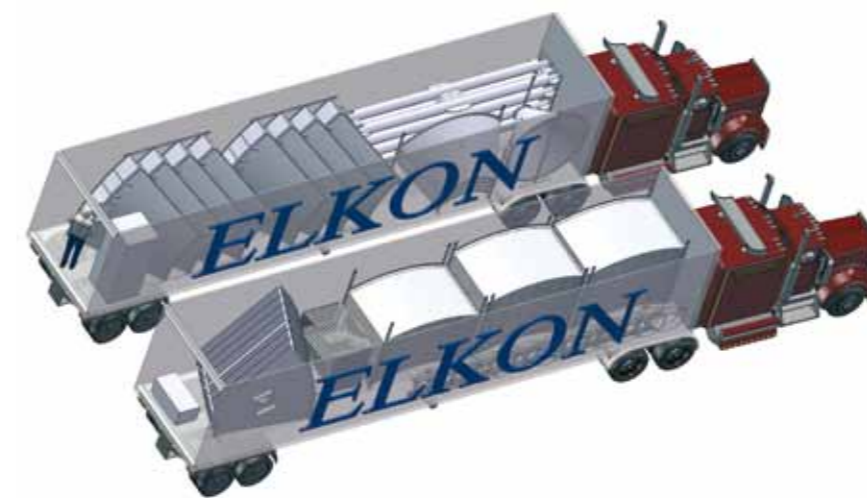
ELKON 500 TONS Bolted Type Cement Silo Container Transportation Scheme
